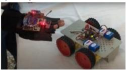
Door Intrusion Detection System – By Shaikh Shahid It is a home security system. It detects intrusion by allowing security check via passcode and RFID card
